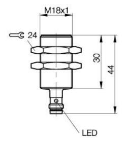
Inductive Sensors BES 516-366-G-E5-Y-S 49 M18x1 x 44 normally-closed Sn=8mm shielded
